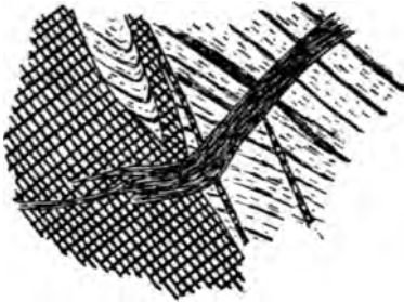
FIG. 2 ( \frac{1}{125} ). — Granite-gneiss dyke cutting banded gneiss and pegmatite (cross-hatched). One branch of the pegmatite has been introduced along a limb of a fold. The pegmatite shows no appreciable foliation, but in the granite-gneiss dyke there is a foliation about parallel to the sides. About 1000 yards S.S.W. of the head of Loch a' Gharbh Bhaid Mhòir.
